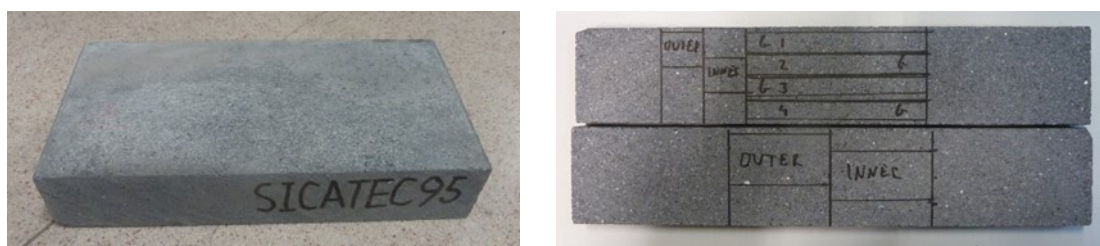
Figure 3. Full size block and sampling positions from the cut surface.
