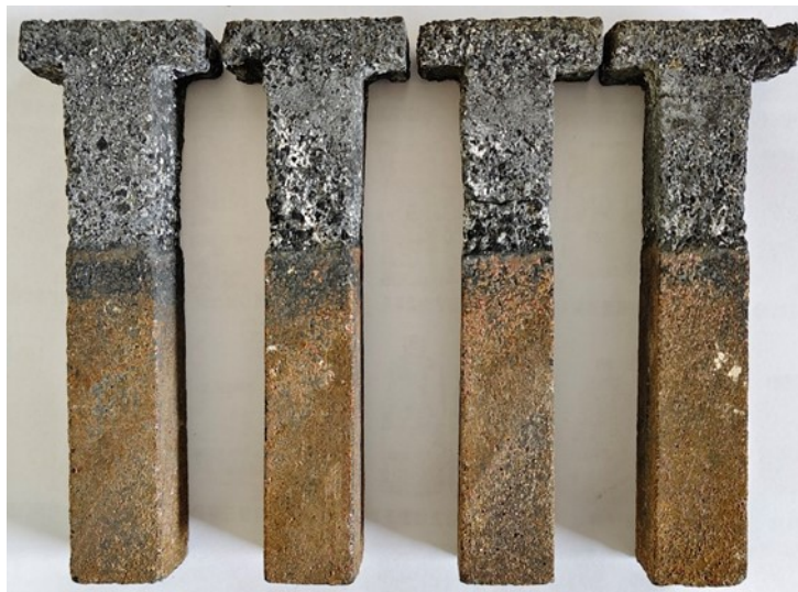
Figure 14. Tested samples after the LIRR test.
